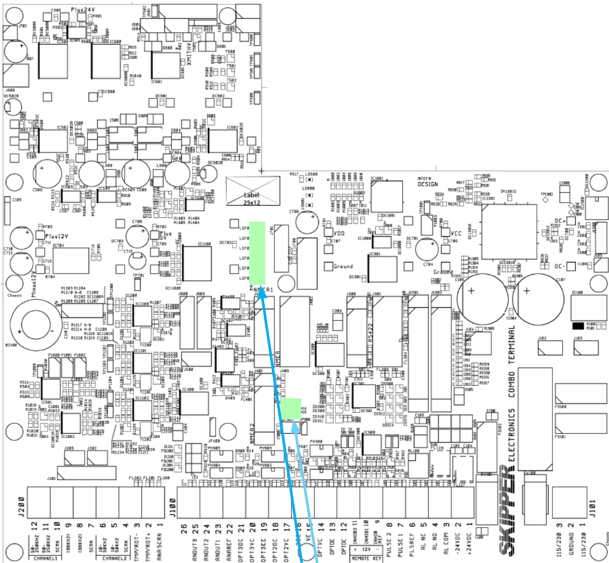
Fig. 4.3 Function LEDs, on terminal board
